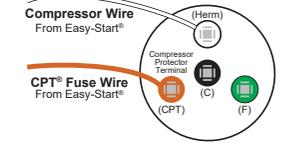
Connect the CPT® Fuse Wire from the Turbo Easy-Start® to the Compressor Protector Terminal® (CPT®) of the AmRad motor-run capacitor.
