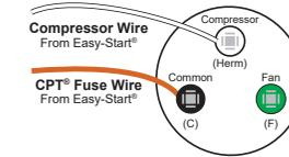
Connect the CPT® Fuse Wire from the Turbo Easy-Start® to the Common (C) terminal of the standard motor-run capacitor.
