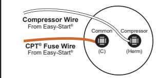
Connect the CPT® Fuse Wire from the Turbo Easy-Start® to either one of the terminals of the motor-run capacitor.
