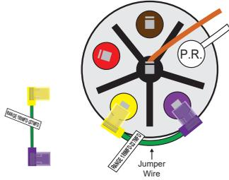
Using the green jumper wire, connect the purple and yellow terminals to the corresponding colored terminals on the Easy-Start® as shown.
