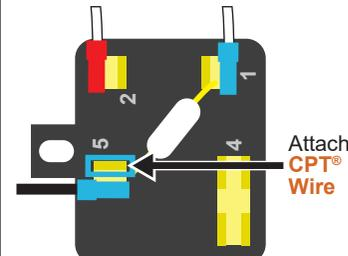
Attach the CPT® Fuse Wire to the indicated terminal (2) on the external relay of the TES5EXT.
