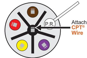
Attach the CPT® Fuse Wire to the white terminal of the TES5.
