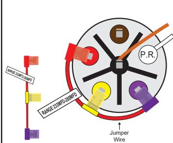
Using the red jumper wire, connect the purple, yellow and red terminals to the corresponding colored terminals on the Easy-Start® as shown.
