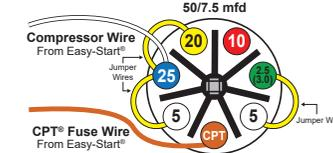
Connect the CPT® Fuse Wire from the Turbo Easy-Start® to the Compressor Protector Terminal® (CPT®) of the Turbo capacitor.
