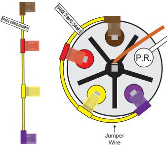
Using the yellow jumper wire, connect the purple, yellow, red and brown terminals to the corresponding colored terminals on the Easy-Start® as shown.
